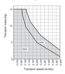
The graph shows total conveyance capacity without accumulating the work.
