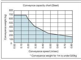
Therefore, it shall be calculated to reduce 2~15% from the chart according to the load
