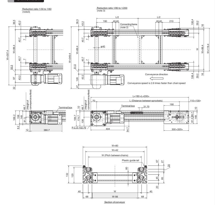
(Note1) The number of <> is size for Distance between sprockets over 3001mm (Note2) When Distance between sprockets is over 2501mm,connecting frame is used in this position (Note3) The motor size is different between Reduction ratio 1/30 to 1/60 and Reduction ratio 1/80 to 1/200
